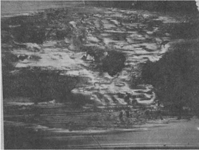
Fig. 1. Wear track of 127- \mu\text{m} DuPont Kapton H polyimide, 90 \times , after 7200 traces of a 1.27-cm diameter 52100 steel slider under a 1-kg load at 24°C, 35% R.H. The average velocity was 15 cm/sec.
