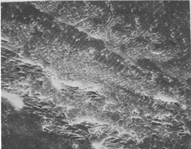
Fig. 2. Wear track of 124- \mu\text{m} Bayer Makrofol N polycarbonate, 500 \times , after 5200 traces of a 1.27-cm diameter 52100 steel slider under a 1-kg load at 24°C, 35% R.H. The average velocity was 15 cm/sec.
